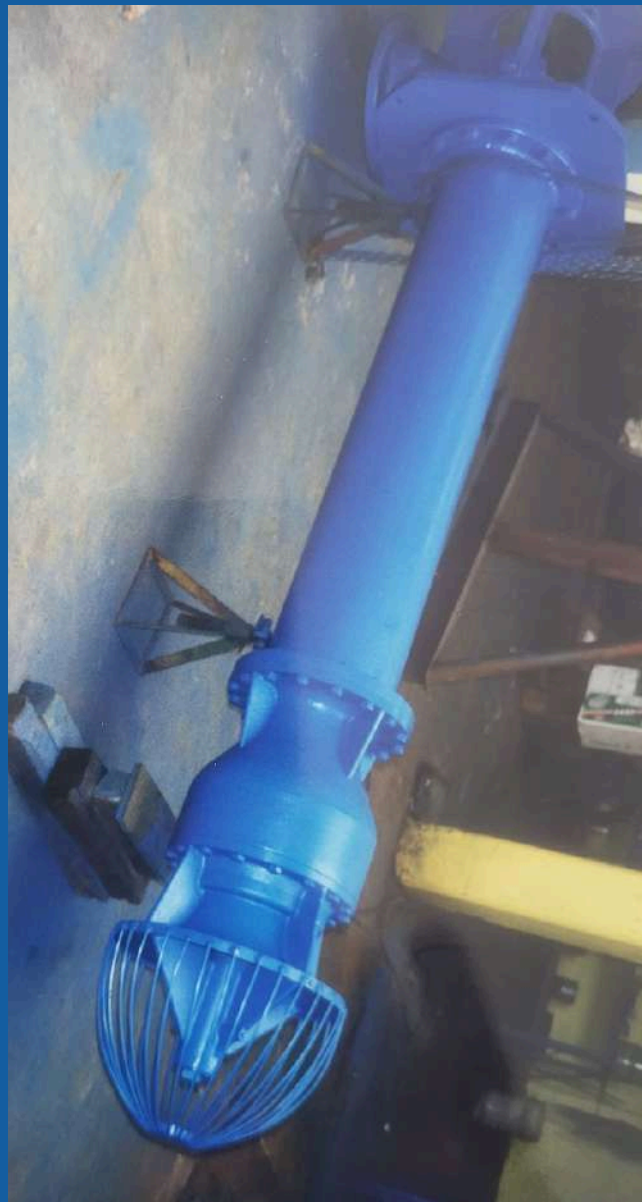
TURBINA VERTICAL 2A 3000 LPS 4 A 56
